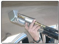
Picture shown HTA-3KM with 4" wide enclosed head for ceiling cleaning
