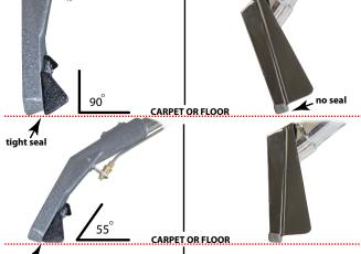
**MAXIMUM SUCTION** when held at different angles NO SUCTION when held at different angles
