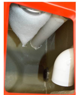
PM10150 wet vacuum filter inside recovery tank
